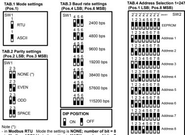
in Modbus ASCII Mode the setting is MARK; number of bit = 7
