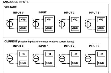
NOTE: the input channels are not isolated between them (terminal GND is common)
